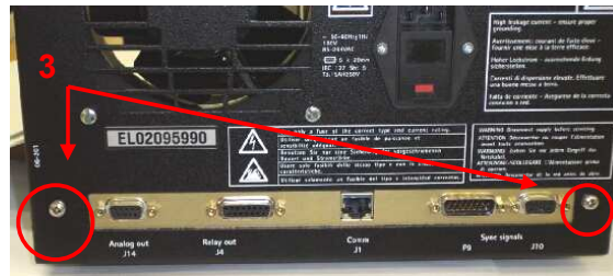
Figure 3: Removing the Screws from the Back of the Detector
